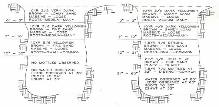
PROBE #6A = 2.4' DEEP PROBE #6B = 1.7' DEEP PROBE #6C = 1.9' DEEP PROBE #6D = 1.6' DEEP PROBE #6E = 2.9' DEEP PROBE #6F = 2.3' DEEP
